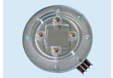
Prototype of a voice coil actuator for image stabilization
