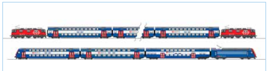
“Refit” the first generation of double-decker railway carriages for the Zurich rapid transit railway system; integration of a new low-floor intermediate carriage (top) and a double-decker train for rush hour traffic (bottom)
