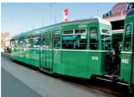
Refurbishing older Type B4 vehicles operated by the Basel Tram Services to make them suitable for disabled persons and reduce noise emissions
