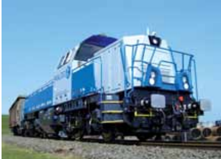
Diesel hydraulic shunting and line locomotive Gravita® 10BB with 1,200kW engine output for local and regional goods transportation
