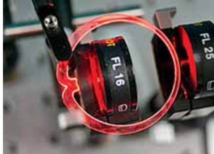
Light guide for bi-directional datalink in optical collector (Stator-Rotor)
