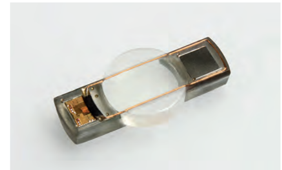
Demonstrator of an accommodating intra-ocular lens (A-IOL) for cataract patients
